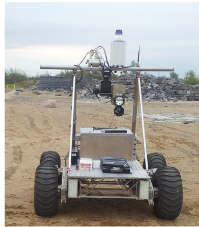
Figure 1. IVIGMS LIDAR (white box on top of the rover mast) on the Juno rover at CSA Mars Yard in 2012.
