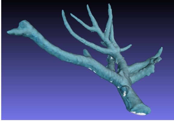
Fig. 10. Final 3-D reconstruction of the piece of Staghorn coral from the multi-view, underwater image dataset.
