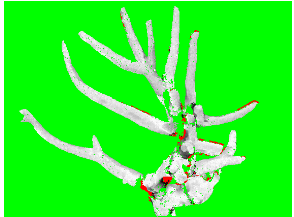
(b) Gathered error statistics: green denotes no ground-truth measure, red a gross error ( > 10\sigma ), white no error increasing towards black ( 10\sigma ).
