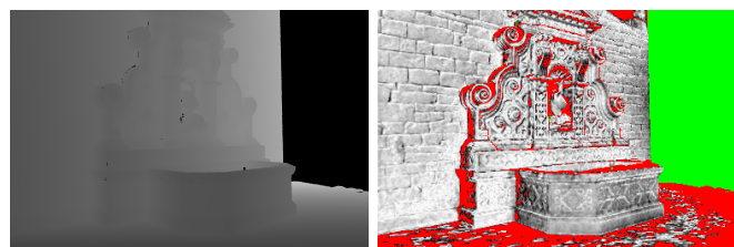
(a) Example image of the rendered (b) Gathered error statistics: green ground-truth depth-map for the fountain sequence. denotes no ground-truth measure, red a gross error (> 10 \sigma ), white no error increasing towards black (10 \sigma ).
