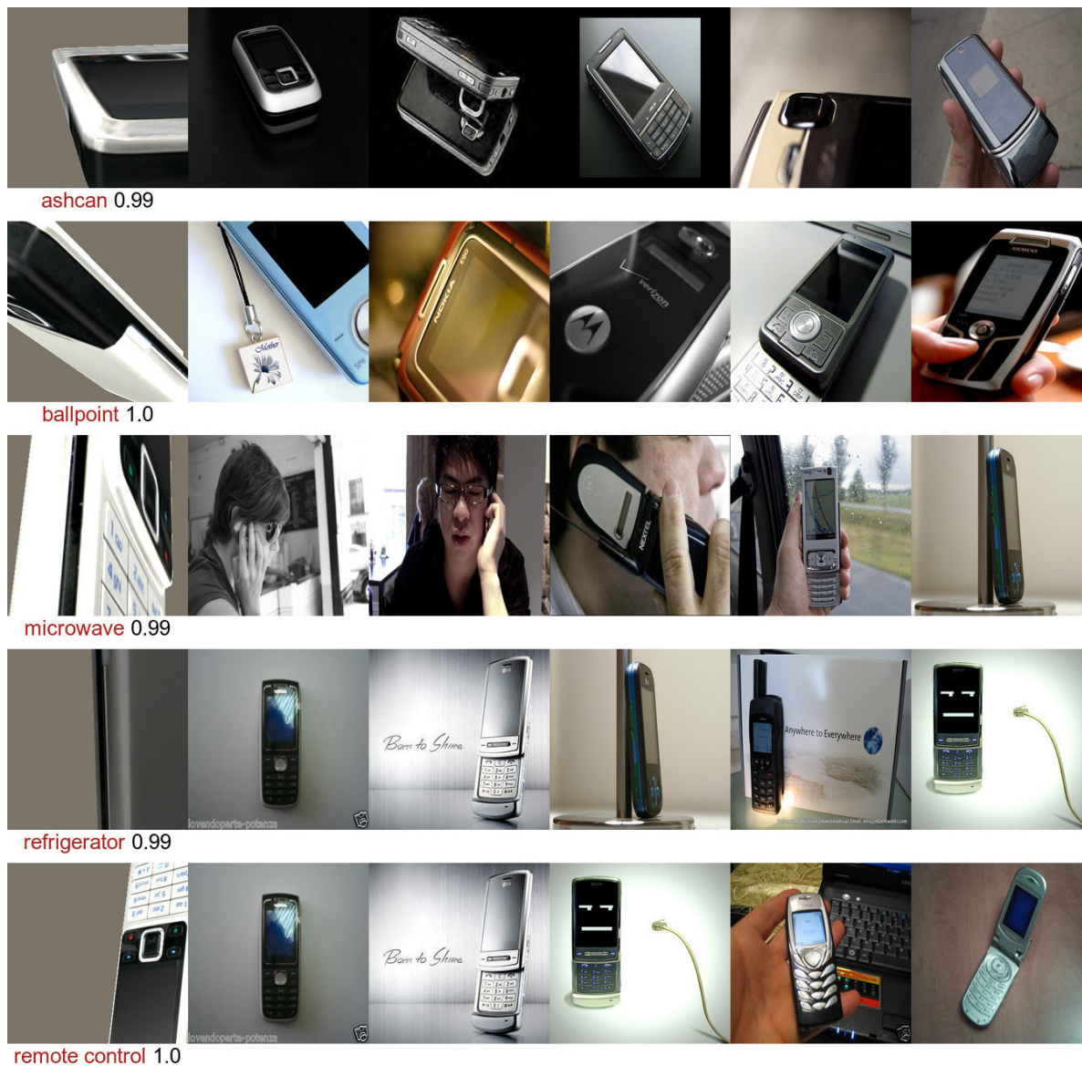
Figure S11: For each adversarial example (leftmost), we retrieved the five nearest neighbors (five rightmost photos) from all \sim 1,300 images in the cellular phone class. The Euclidean distance between a pair of images was computed in the fc7 feature space of a pre-trained AlexNet [20]. The nearest photos from the class are mostly different from the adversarial poses. This result supports the hypothesis that the generated adversarial poses are out-of-distribution. The original, high-resolution figure is available at https://goo.gl/X31VXh .
