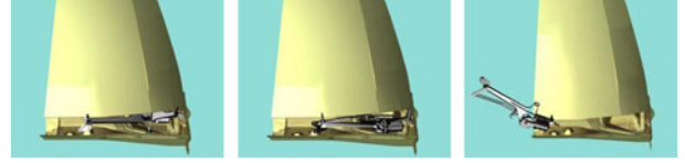
Fig. 8. Three image shots that show animation sequences of getting a wiper out of the windscreen model. Since there are not much rooms between two models, this benchmark has narrow passages.
