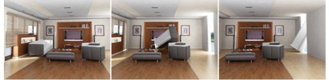
Fig. 1. Living room benchmark: This figure shows three image shots of getting a sofa out through a door, which creates narrow passages in 6-degrees-of-freedom (DoFs) configuration space. Our method achieves ten and two times improvement over a basic RRT and an optimization-based retraction method, respectively.
