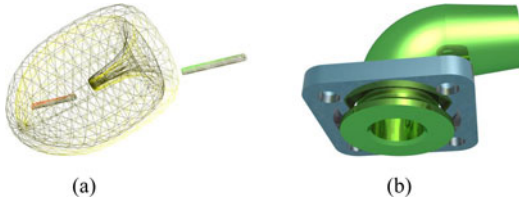
Fig. 7. Two different benchmarks that have narrow passages. Note that a robot of a bug-trap benchmark is initially located outside of a trap. (a) Bug-trap. (b) Flange.
