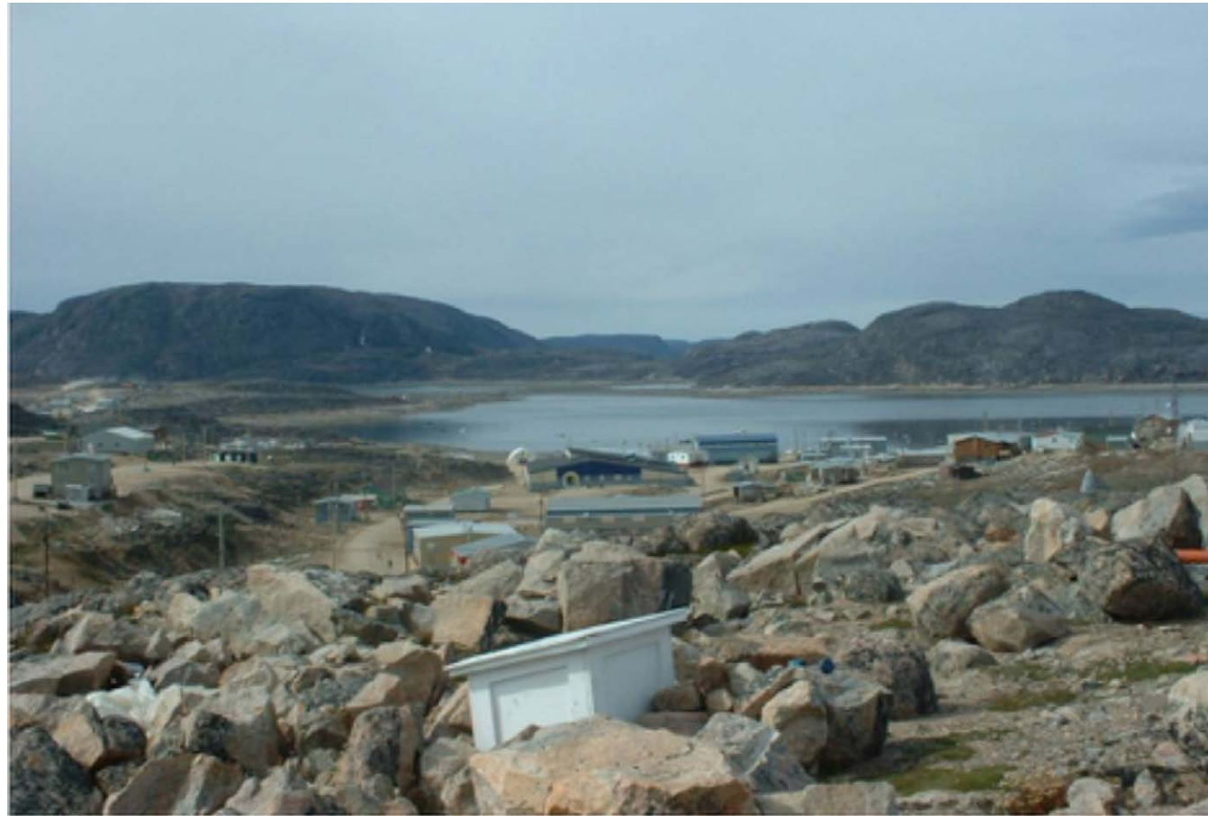
Figure 7. MACCS magnetometer sensor (inside the white box) at Cape Dorset during Arctic summer. MACCS consists of two approximately east-west chains at 75° and 80° north geomagnetic latitude in eastern Arctic Canada. Each system is located at an Inuit village (often near the airport, as at Cape Dorset, or other public infrastructure facility) where power and local volunteer support can be provided. MACCS data were originally recorded on tape cassettes mailed to the U.S. monthly; currently data are transmitted in near real time via village wireless internet, or in two cases via the Iridium satellite telephone system.
