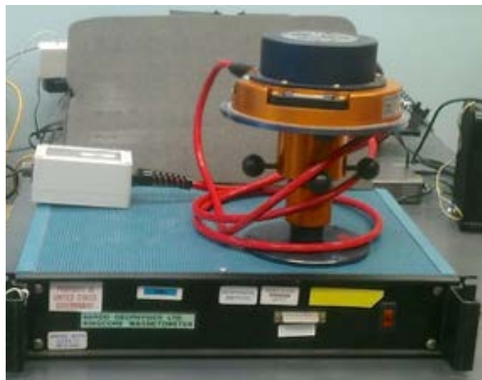
Figure 5. Narod fluxgate magnetometer sensor (top) and controller (bottom): These instruments are used by the USGS, GIMA (Alaska), and MACCS arrays.
