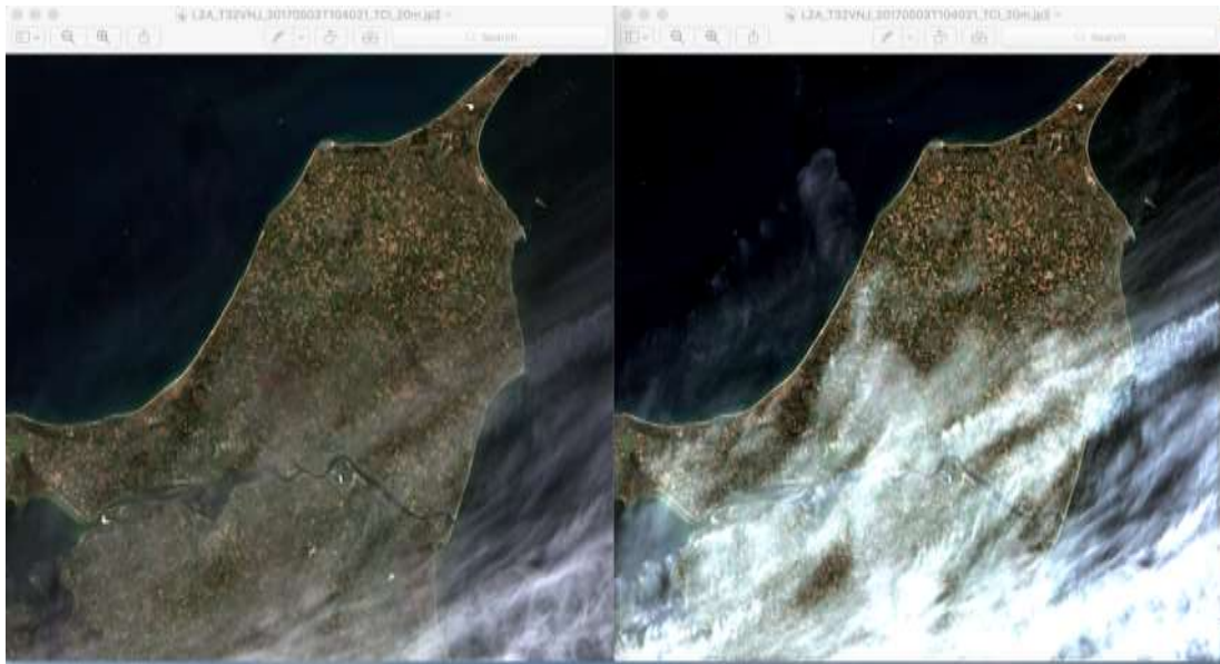
Figure 2-11 – Cirrus Correction over north Denmark, Bands 2-4 with Band 10. Left: L2A Output cirrus corrected, right: without correction.
