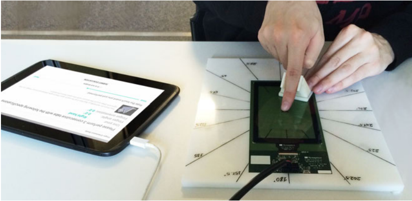
Figure 4.3: The apparatus we used in our study, showing the tablet, the touch layer and one of the pitch stabilizer while one participant touches the touch surface.
