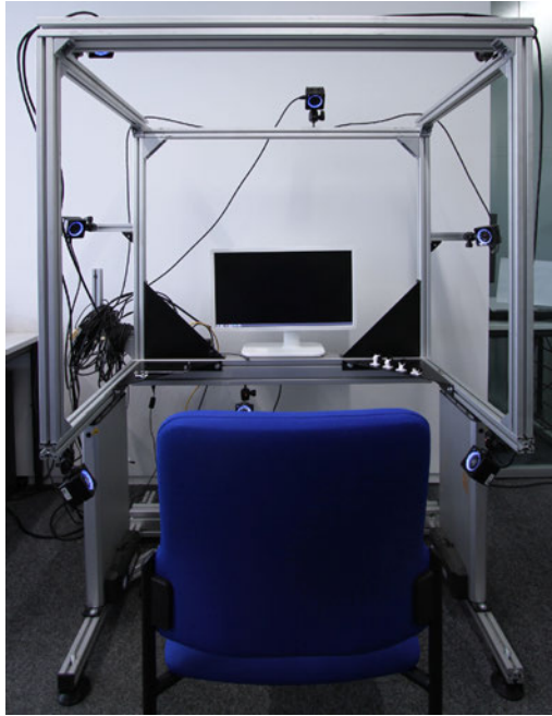
Figure 4.9: The setup with the 6DOF tracking system, the four pitch stabilizer on the left and the Motorola Nexus 6 with markers.
