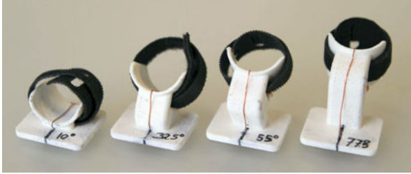
Figure 4.11: (a) The four pitch stabilizers with the copper plate and the wire, we used in the study to limit PITCH to 77.5^\circ , 55^\circ , 32.5^\circ and 10^\circ presented from left to right. (b) A CAD model of a pitch stabilizer, revealing the wiring and the copper plate in the base.
