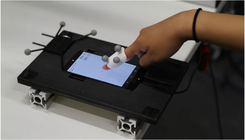
Figure 3.7: A close up of a participants hand while performing the study. On the participants index finger we attached the ridget body to track the finger orientation.
