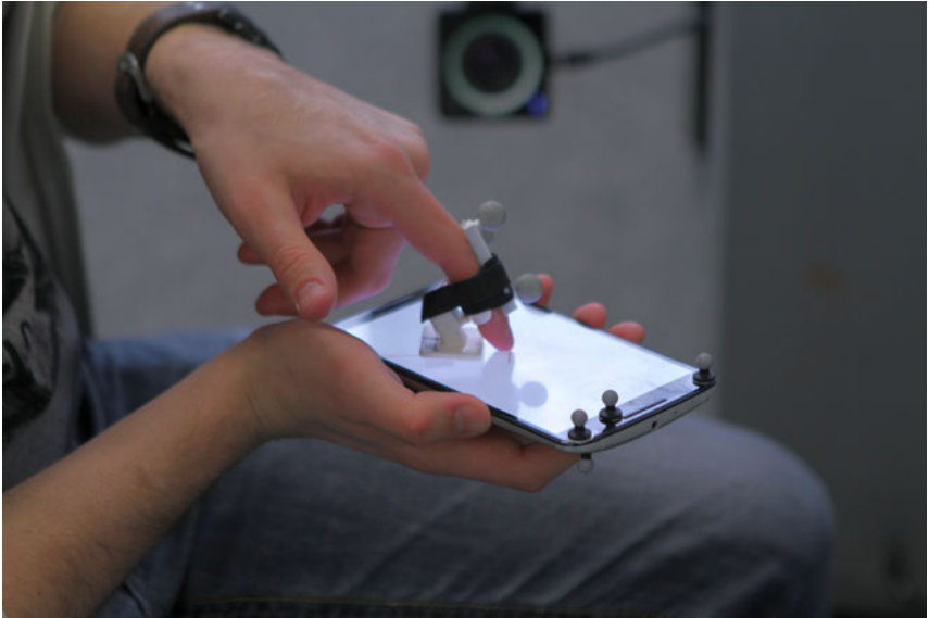
Figure 4.8: A participants performing a 32.5^\circ pitch and 45^\circ yaw input with the left hand while being equipped with our 3D printed tracking parts.
