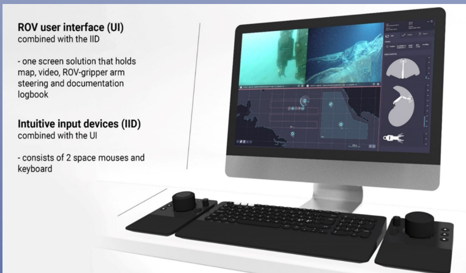
Final prototypes of SWARMs intuitive input device and ROV user interface
