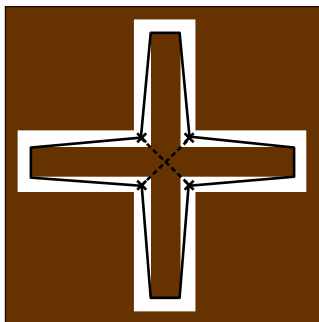
Figure 6: A worst-case example for LAZY-GMGP in a two-dimensional configuration space C . The free space F is shown in white and each of the 4 cross-marks denotes a goal configuration. The dashed and plain lines depict the shortest paths between the goals in C and in F , respectively. The length of the shortest path in C between any two goals is much smaller than the length of the shortest path in F between any two goals.
