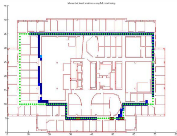
Fig. 5. The performance of the positioning algorithm using deterministic parameters. The green dots lie on the actual trajectory taken by the mobile and the blue squares represent the estimated trajectory. The estimated trajectory is color-coded to indicate the reliability associated with the estimated position as reported by the algorithm: the darker the color, the higher the reported reliability. The key point is that inaccurately estimated positions are reported as reliable by the algorithm, which is an artifact of model error.
