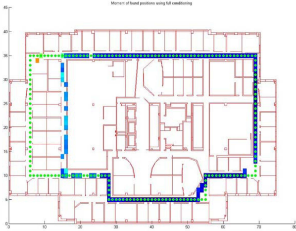
Fig. 6. The performance of the positioning algorithm using stochastic parameters. In particular, the five global parameters are considered to be independent and uniformly distributed on a wide support. The key point to note is that the inaccurate position estimates are detected by the algorithm and labeled with low reliability metrics (the light-blue positions).
