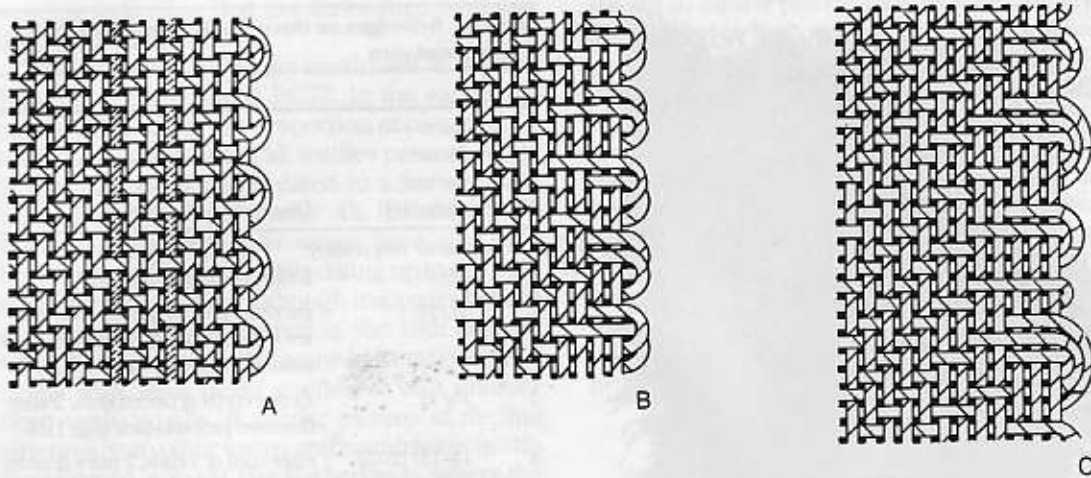
Fig 11 Selvedges on three-shed twills woven from Z-spun yarn: (A) No 2, (B) No 3, (C) No 4
