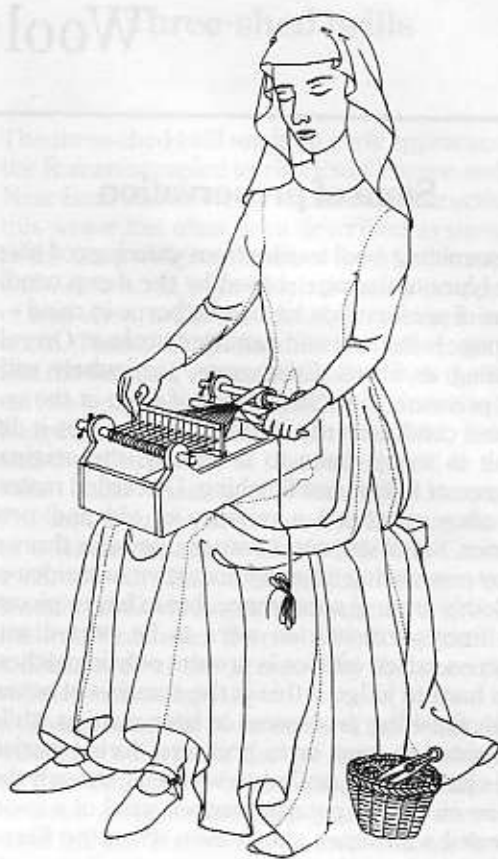
Fig 8 Box loom with a rigid heddle as it might have looked in the 14th century
