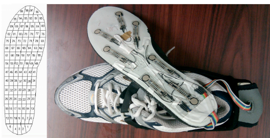
Figure 1: Right: medical shoe instrumented with pressure sensors. Left: pressure sensor location map under the foot for Pedar’s insole. Sensor placement and location are derived from studying Pedar’s insole, which has 99 sensors
