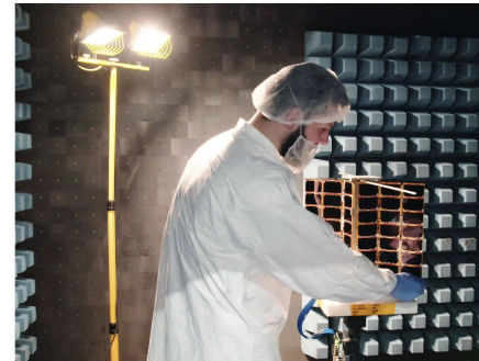
An engineer at Spire, a smallsat company that got a NOAA contract in 2016, prepares a satellite for antenna testing. © SPIRE
