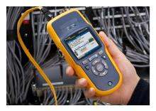
to blame. If connectivity issues are resolved by connecting to the router, then you will need to backtrack through the system to determine if there is a faulty patch cable or horizontal cabling along the network path.
