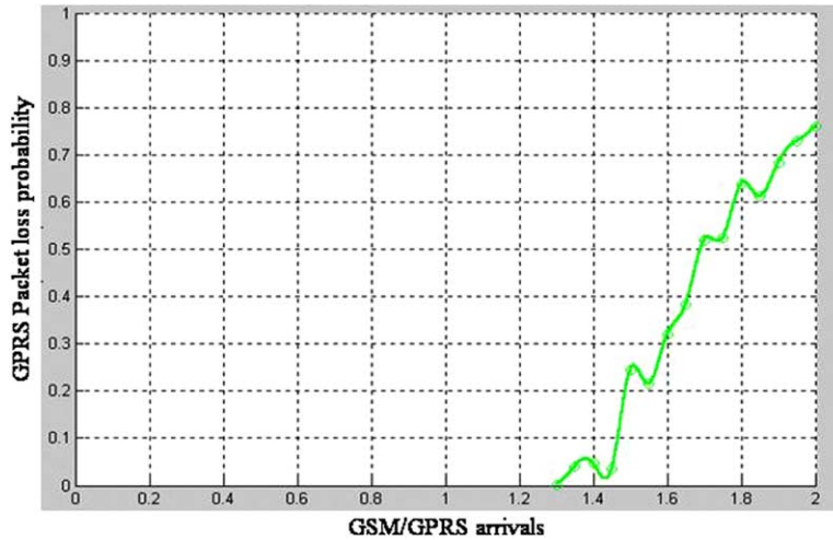
Fig. 13. Packet-loss probability in the dynamic allocation scheme.
