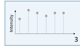
(c) The mean intensity of each slice is computed and stored with its local position x within the voxel.
