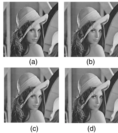
Figure 2. Coding results for test image 'Lena': (a) Original; (b) 0.1892 bits/pixel, 29.3270 dB; (c) 0.2666 bits/pixel, 31.4672 dB; (d) 0.4540 bits/pixel, 33.4164 dB.
