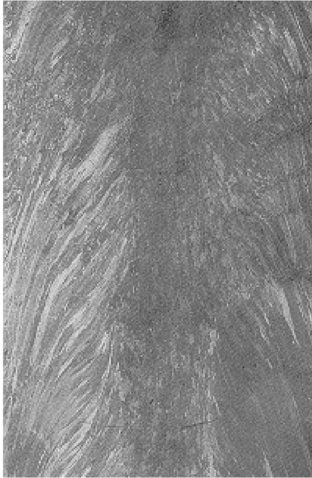
Figure 10: Grain structure of a non grain refined 178 mm diameter billet.
