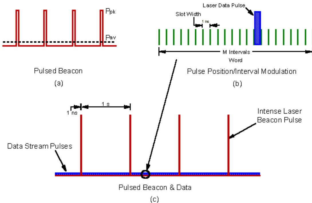
Figure 6. A scenario for pulsed laser beacons and wideband data signals that might be produced by an ETI civilization. This would make for easier detection in the presence of stellar background radiation, and the precise "magic laser wavelength" need not be known.
