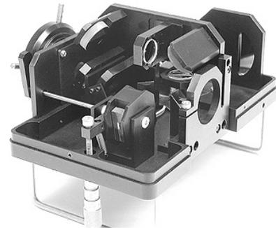
Figure 5. Santa Barbara Instrument Group's (SBIG) Self-Guiding Spectrograph for use with their ST-7E CCD camera.<sup>h</sup>
