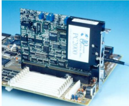
Figure 4. Ocean Optics Fiber Optic Spectrometer.<sup>g</sup>
