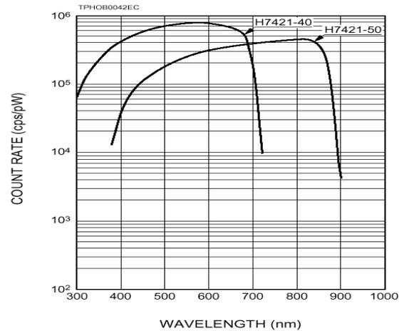
Figure 13. Spectral response for the Hamamatsu H7421 PMT Photon Counter.
