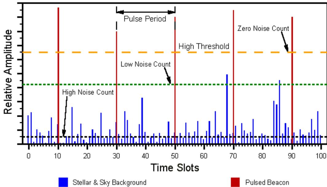
Figure 10. When employing a single photon-counter, the background noise can be reduced by setting the discriminator level higher than normal. This amounts to a desensitization of the receiver, but if the ETI beacon pulses are expected to be relatively intense, then this is a reasonable approach for substantially reducing the background count. If a burst of beacon pulses is expected, then this simple and lower cost form of receiver could be adequate for the task.
