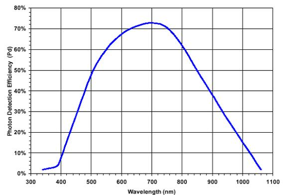
Figure 15. Spectral response for PerkinElmer SPCM.
