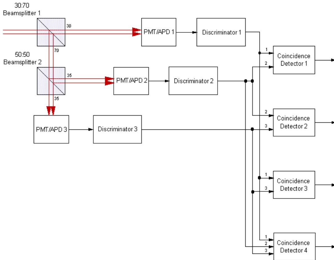
Figure 16. An extension of the coincidence system of Figure 11, but employing three photon detectors. This system is described elsewhere in these proceedings.<sup>44</sup> A system based on this technique is being installed at the Lick Observatory.
