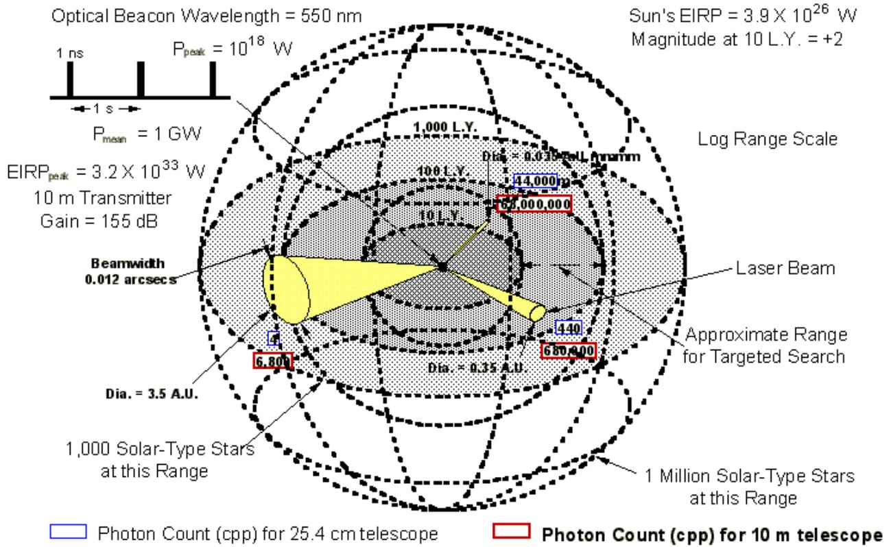
Figure 7. Signal photon detection rate for small and large ground-based telescopes assuming a very conservative overall photon detection efficiency of one percent. Under this scenario, there would be no problem for amateur telescopes in detecting 1 ns laser pulses of  $10^{18} \text{ W}$  peak power over a range of 1,000 light years.
