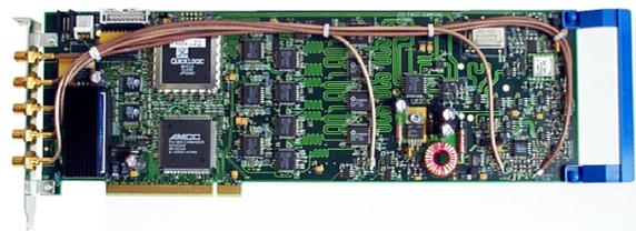
Figure 18. FastComTec ultra-fast P7886 2 GHz Time-of-Flight/Multiscaler.
