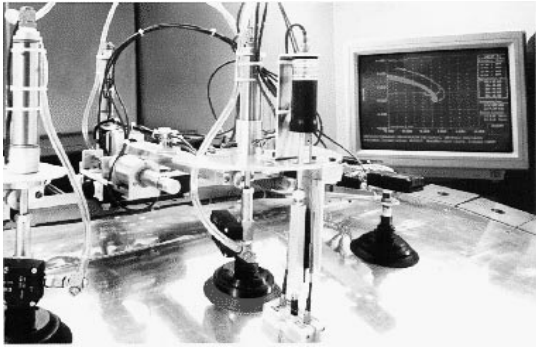
Fig 1. Automated NonDestructive Inspection (ANDI) robot
