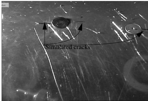
Fig 6a. Metal surface with three synthetic cracks and other crack like features
