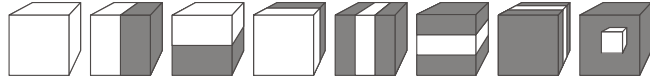
Fig. 2. Volumetric Haar-like filters used to extract features for mitosis detection. The features are computed by subtracting the sum of pixel values in the black boxes from the sum of pixel values in the white boxes.
