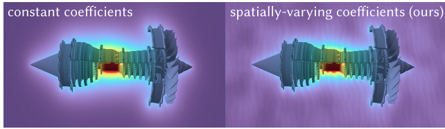
Fig. 2. We directly resolve the detailed effects of, e.g., spatially varying material density—without resorting to homogenization of PDE coefficients.
