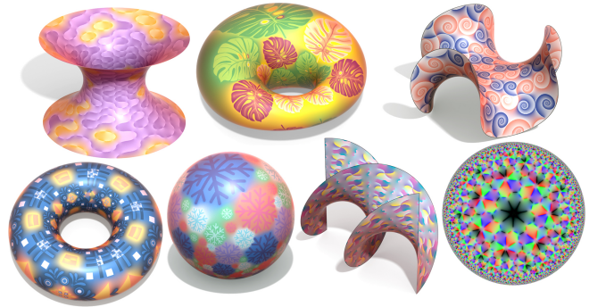
Fig. 21. Variable coefficients enable us to extend WoS to curved domains (not previously possible). Here we directly resolve intricate boundary conditions for diffusion curves—without generating a fine surface mesh that conforms to boundary curves or a spatially-adaptive grid in the parameter domain.
