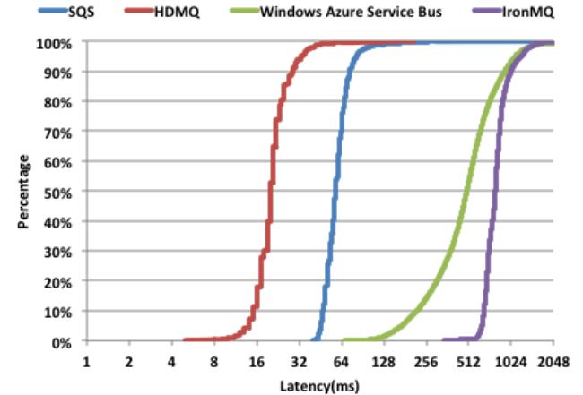
Figure 9 Comparison of HDMQ, SQS, Windows Azure Service Bus, and IronMQ with 64 KB message Size
