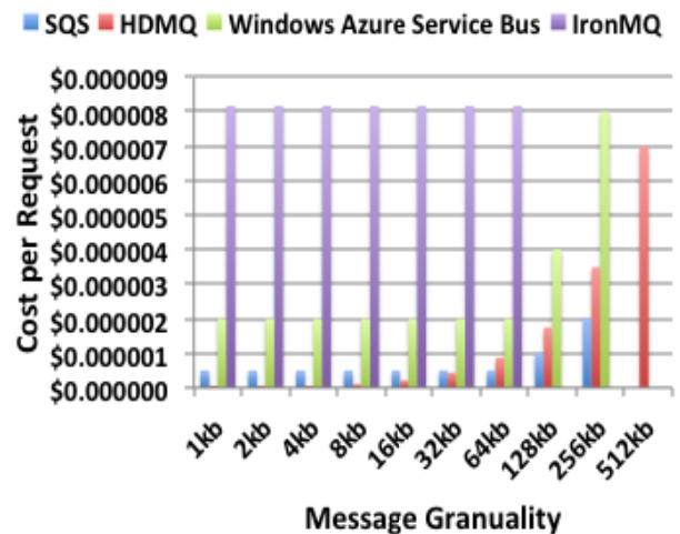
Figure 15 Cost per Request HDMQ vs. SQS
