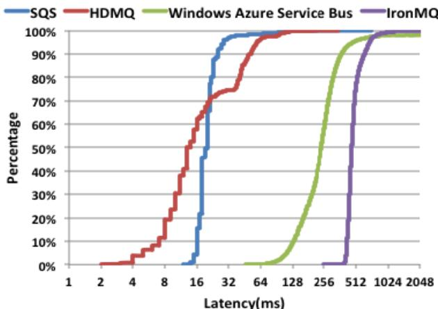
Figure 7 Comparison of HDMQ, SQS, Windows Azure Service Bus, and IronMQ with 1 KB message Size
