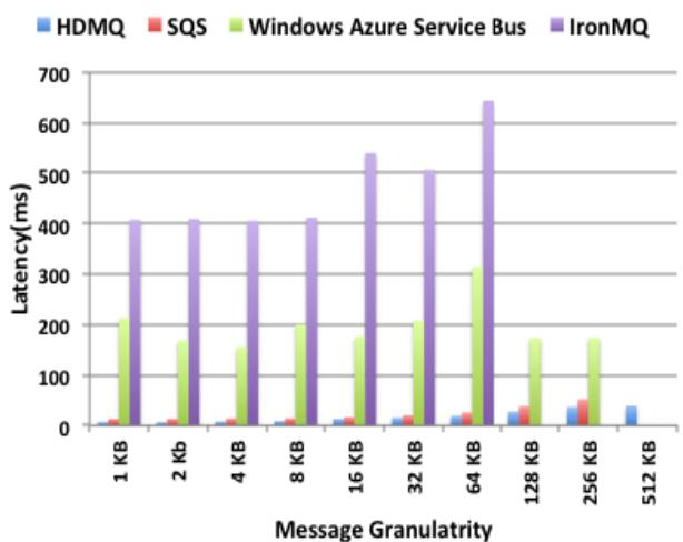
Figure 11 Average Latency HDMQ vs. SQS vs. IronMQ vs. Windows Azure Service Bus for Retrieving Message
