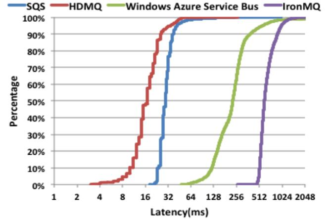
Figure 8 Comparison of HDMQ, SQS, Windows Azure Service Bus, and IronMQ with 16 KB message Size
