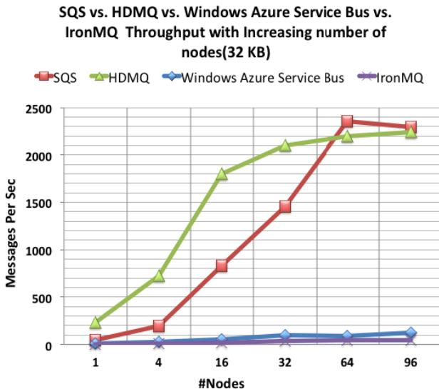
Figure 14 Throughput with increasing number of nodes with message size 32KB for HDMQ, IronMQ, Amazon SQS and Windows Azure Service Bus
