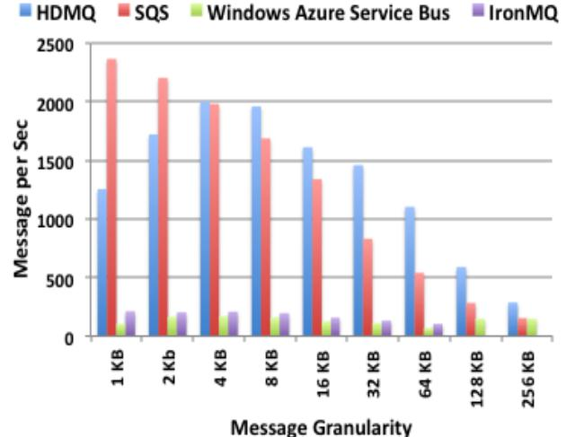
Figure 12 Message Adding Throughput HDMQ vs. SQS vs. IronMQ vs. Windows Azure Service Bus
