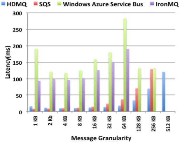
Figure 10 Average Latency HDMQ vs. SQS vs. IronMQ vs. Windows Azure Service Bus for Adding Message
