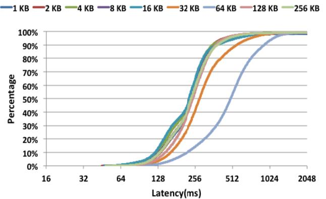
Figure 5 Windows Azure Service Bus System Latency
