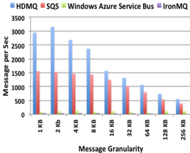
Figure 13 Message Adding Throughput HDMQ vs. SQS vs. IronMQ vs. Windows Azure Service Bus
