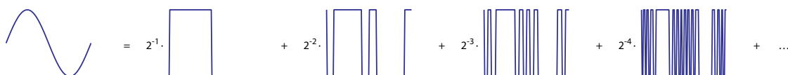
Figure 13: A projector illuminates the scene with a sinusoidal pattern, and a camera takes the corresponding photo. Multiple photos at various exposures capture high dynamic range images to produce photos with high bit-depths. If the projector pixels have binary values, the sinusoidal pattern is subject to severe quantization errors, and same goes for the photographs. By decomposing the signal into a series of binary illumination patterns and collecting their corresponding photos, a weighted sum of the photos produces the correct response. Note that photos with small weights become dominated by the sensor noise of the photos with large weights.
