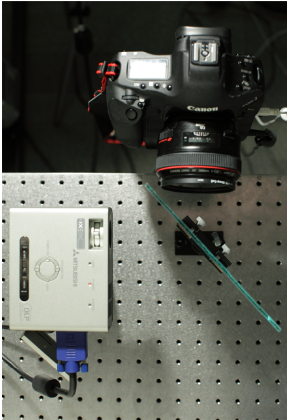
Figure 14: A top-down view of the setup for capturing the eigenvectors of symmetric light transport matrices.
