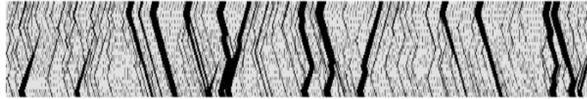
Figure 7. Communication (black) and computation (light gray) times for the 32 threads in the 'one thread per CPU' configuration (one cluster, 8 nodes, 4 CPU's per node).
