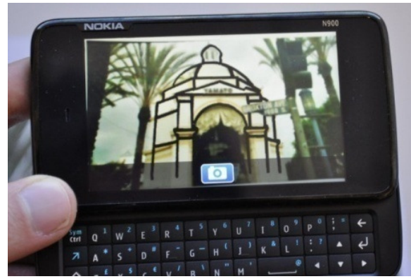
Figure 5: A user holding an N900 and aligning a static outline of the building with the real building behind. This calibration step is used to start the effect at Yamato, and as a backup to start the effect at Peet's.
