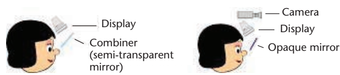
2 Concepts of optical see-through (left) and video see-through displays (right).
