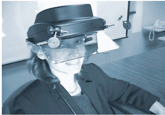
4 Experimental head-worn projective display using lightweight optics. (Courtesy of Jannick Rolland, University of Central Florida, and Frank Biocca, Michigan State University.)
