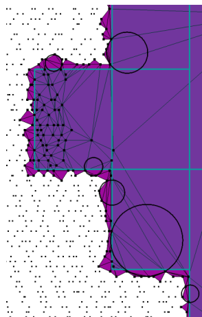
Figure 4: A closeup of streaming Delaunay in 2D. The points on the left have been processed, and their triangles written out. All triangles in this figure are active . We have drawn a few representative circumcircles, all of which intersect unfinalized space. At this moment, points are being inserted into the leftmost cell, which will be finalized next.
