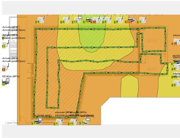
(b) ISM spectrum (namely, WLAN) interference study in the site's area [4].
