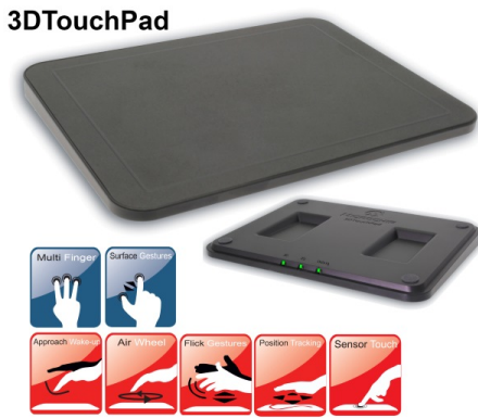
Figure 7: Touch+air gestures acquired by 3D TouchPad. Source: https://www.microchip.com/DevelopmentTools/ProductDetails/DM160225
