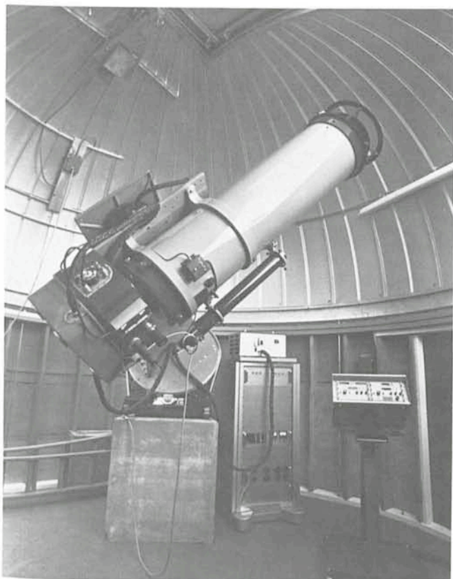
The 40 cm Cassegrain telescope of the Geneva Observatory on La Silla. The photoelectric photometer is at the Cassegrain focus.
