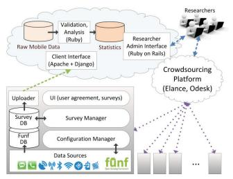
Figure 2: System architecture for the mobile data collection system including a mobile client, a server, and crowdsourcing platform.
