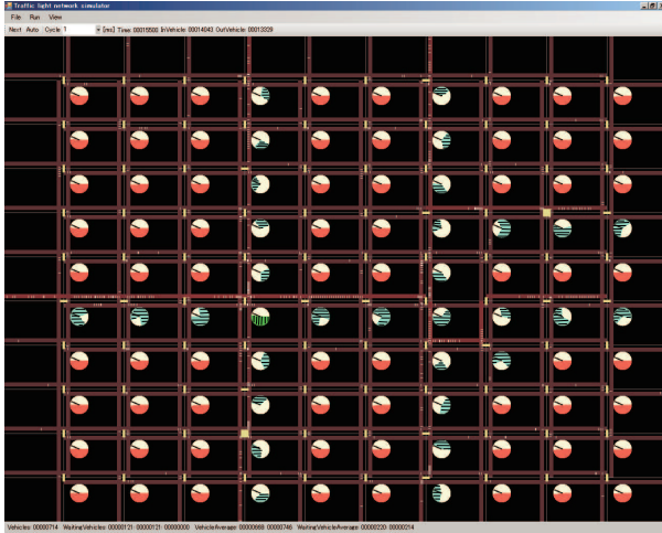
Figure 11: Screenshot of simulator of experiment 4 (New green-wave formation is constructed according to change in traffic flow)
