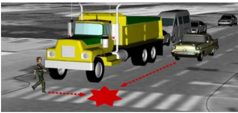
Figure 4: Experimental setup: high truck A is stopped in the lane adjacent to the sidewalk and obscures the view of both the pedestrian and of approaching car B
