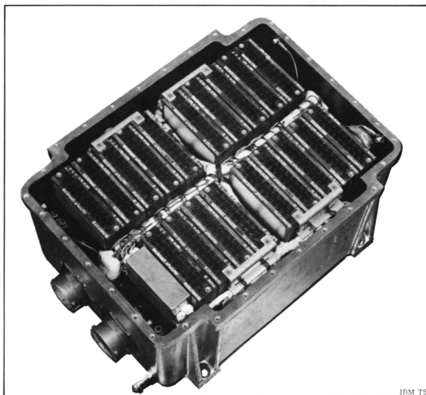
Figure 1-5. Switch Selector, Model II (Internal View)
