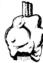
C. EXCESSIVELY SOLDERED JOINT
