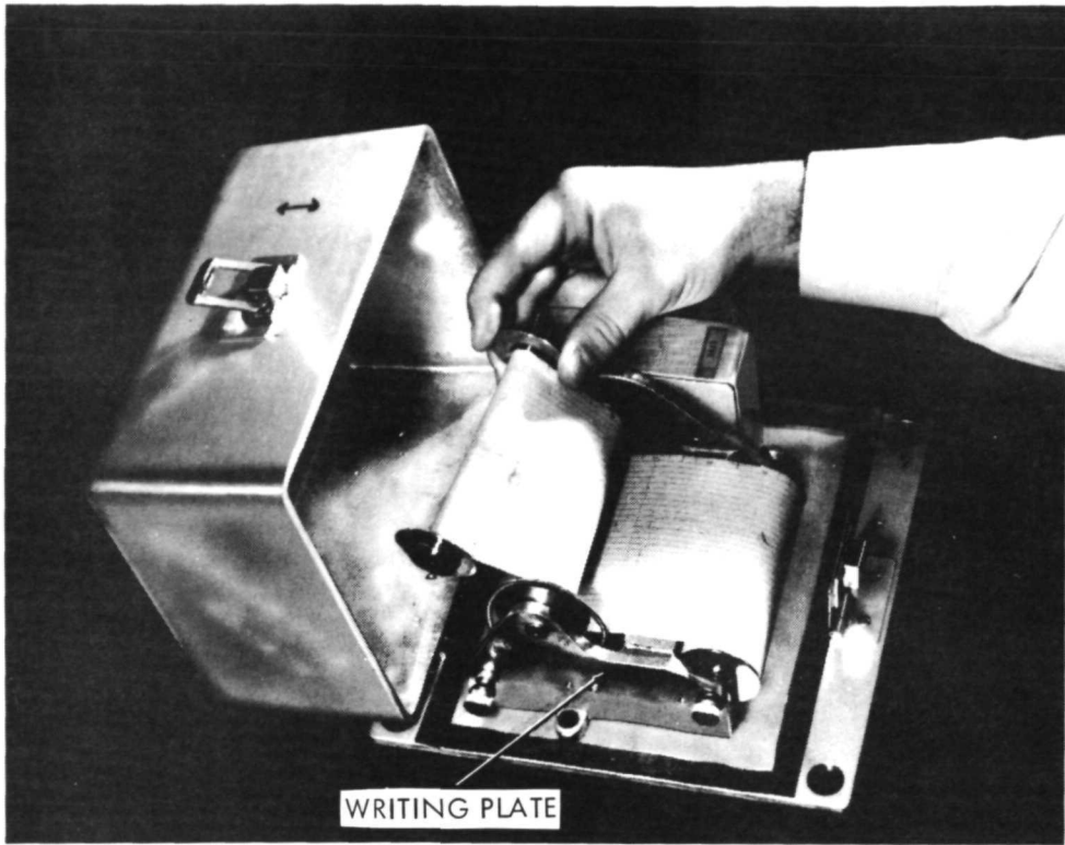
Figure 5-2. Removing Roll Chart From Shock Recorder.
