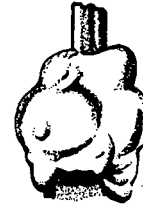
C. EXCESSIVELY SOLDERED JOINT
