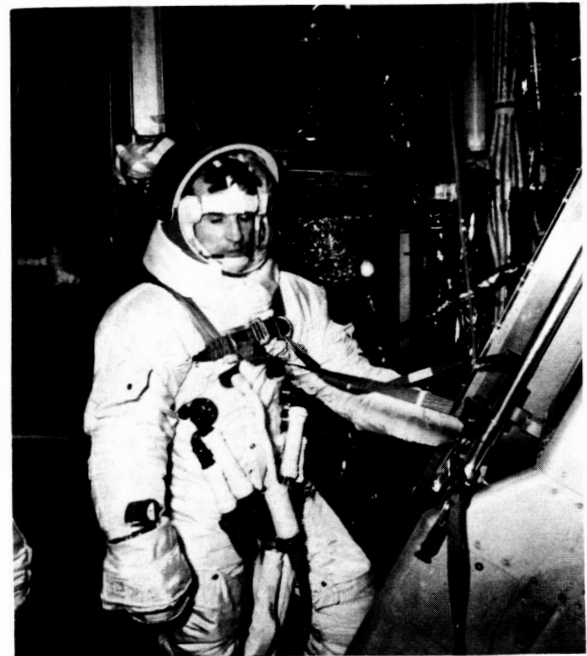
Figure 19. - Falling restraint system and umbilical connections.
