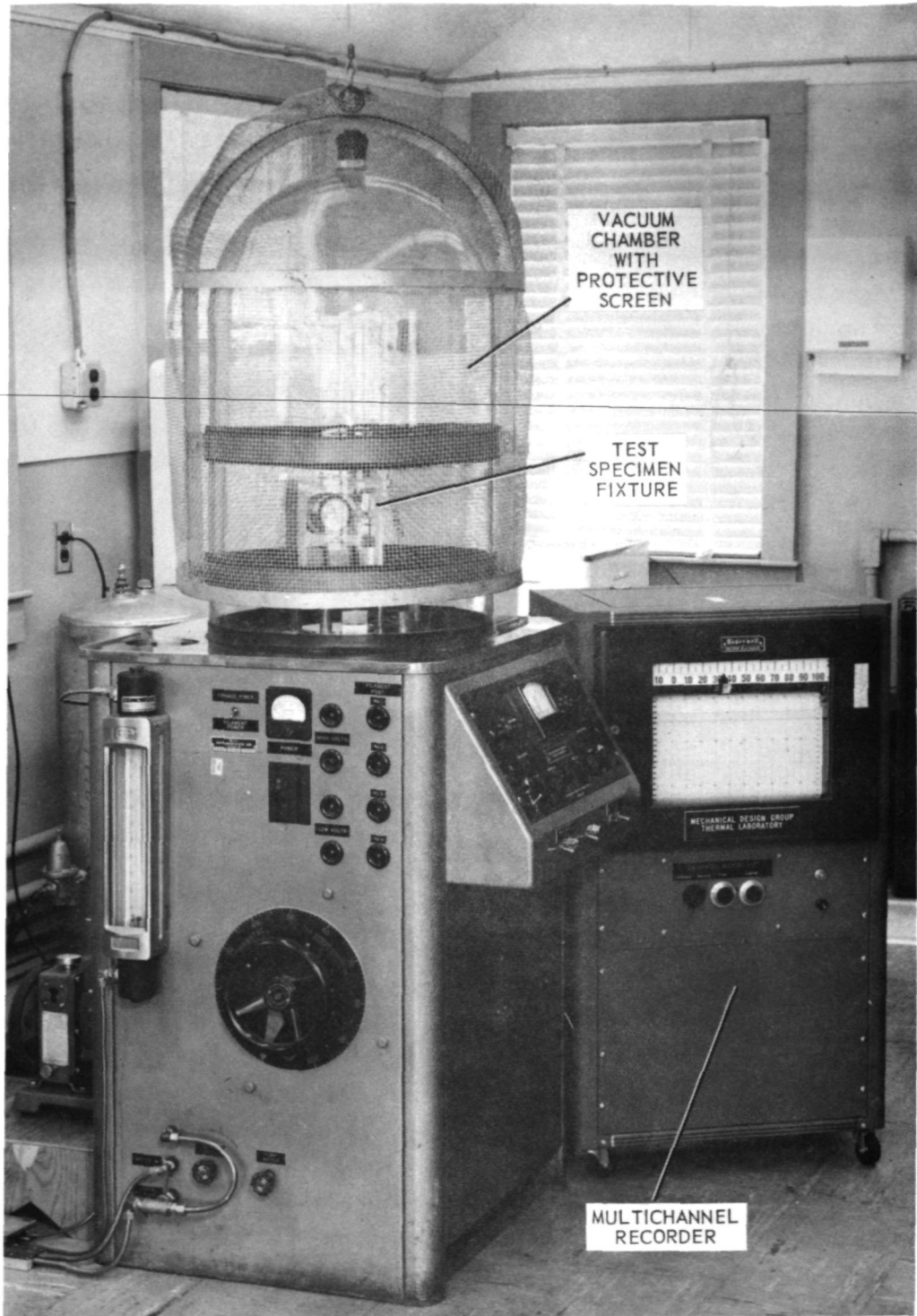
Fig. 1. Equipment setup for high-vacuum heat transfer investigations.
