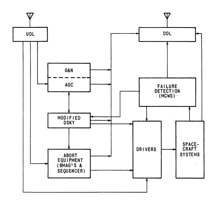
FIGURE I PROGRAMMER FOR UNMANNED SATURN IB MISSIONS
