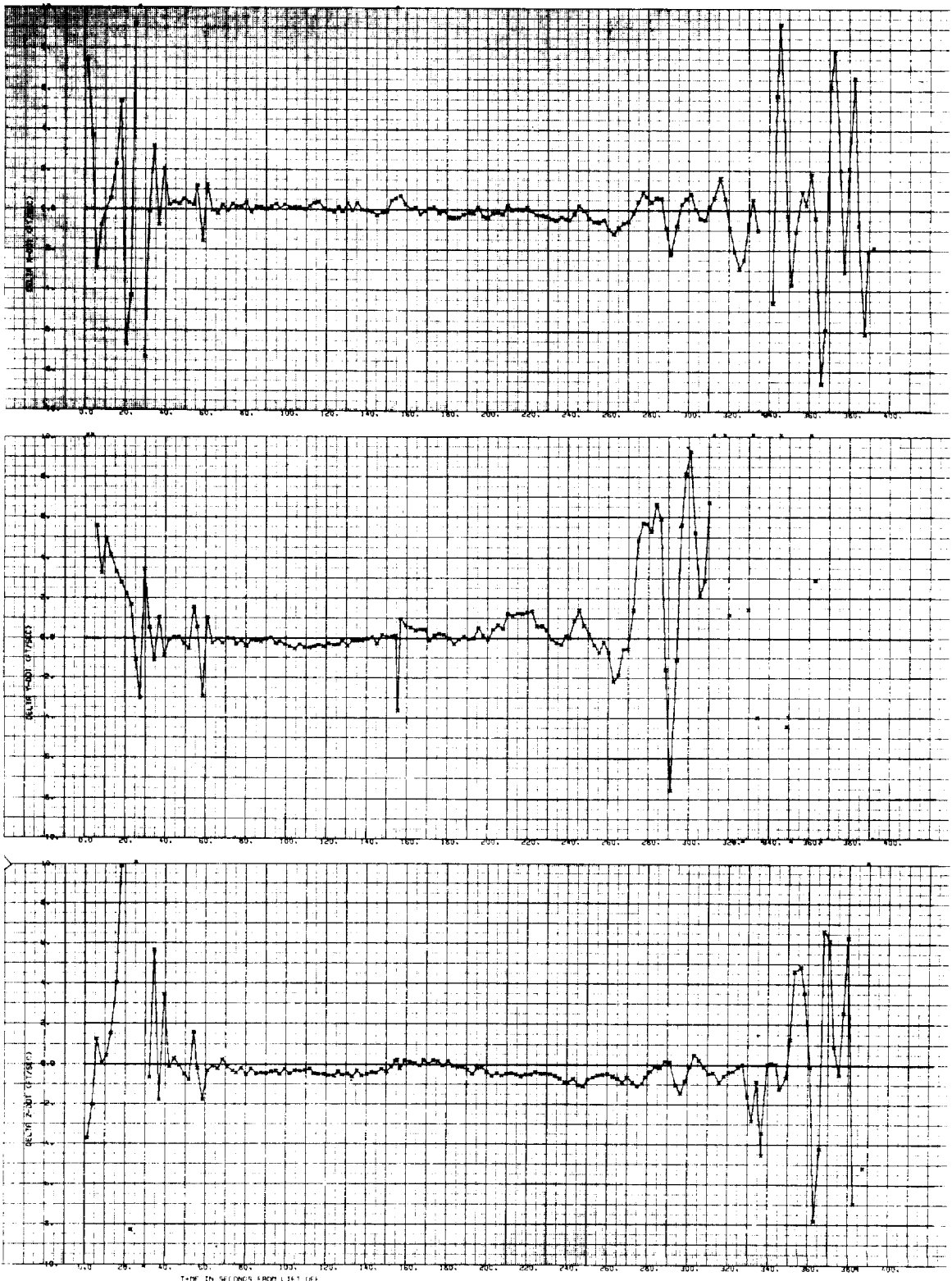
Figure 16. GE/Final Thrust Velocity Comparison with IMU Errors Compensated
