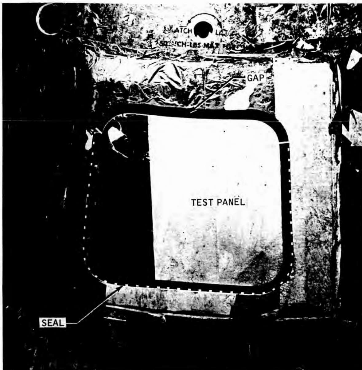
FIGURE 5.4-25.- UNIFIED SIDE HATCH TEST PANEL SHOWING GAP AND SEAL.
