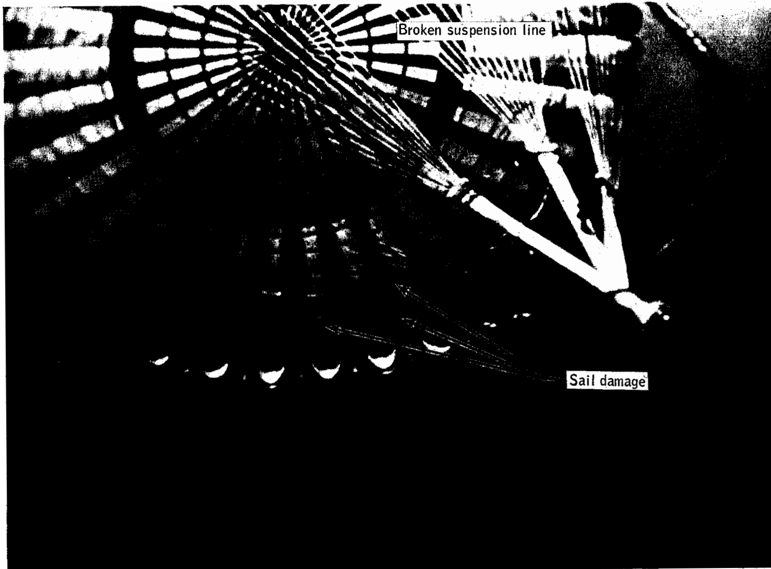
Figure 8.1-6.- Main parachute damage.
