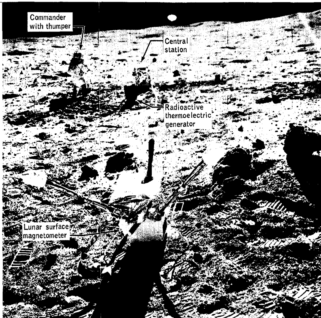
Figure 4-7.- Lunar surface magnetometer experiment and Commander performing active seismic experiment.
