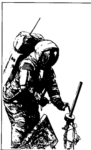
Alignment Of Passive Seismometer
