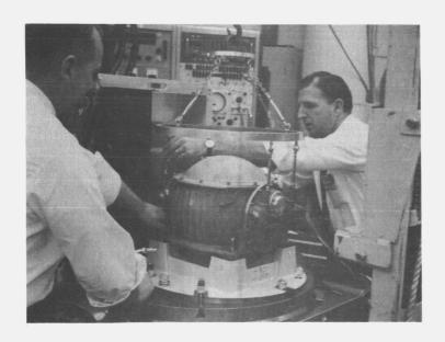
Figure 6. Removing IMU #4 from test fixture.
