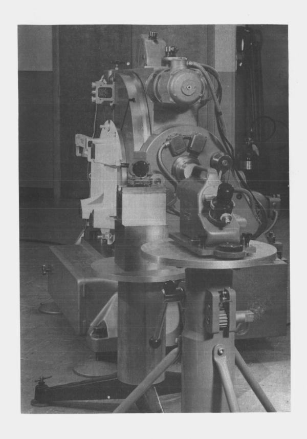
Figure 3. Measuring IMU fixture axis alignment to table - top axes about Z (JDC 0012).
