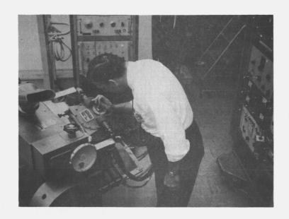
Figure 5. Applying indicator sealant to IMU #4 Resolver Zero Adjustment Module.
