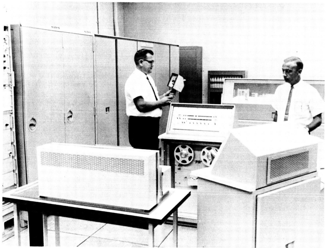
Figure 38. Instrumentation Data Test Station
