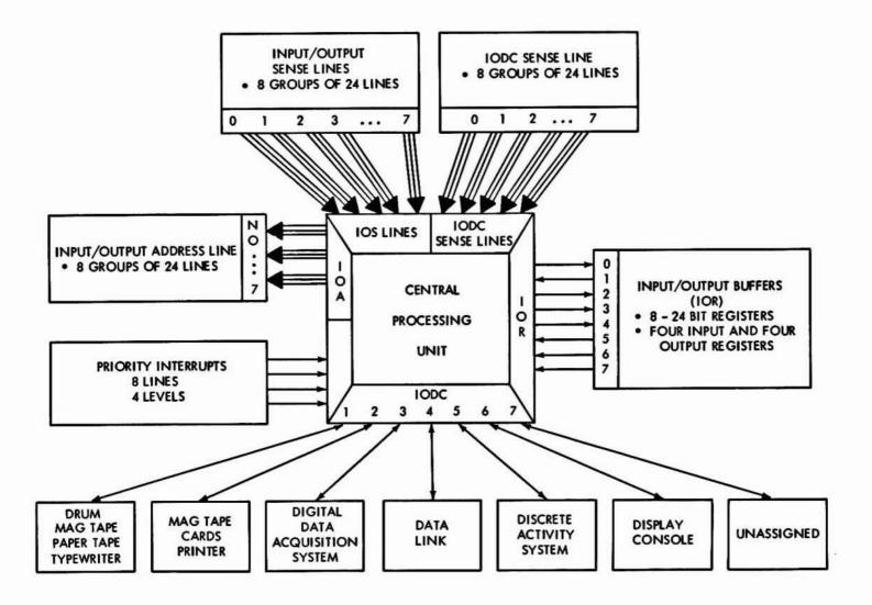
Figure 3. Computer Input/Output System.
