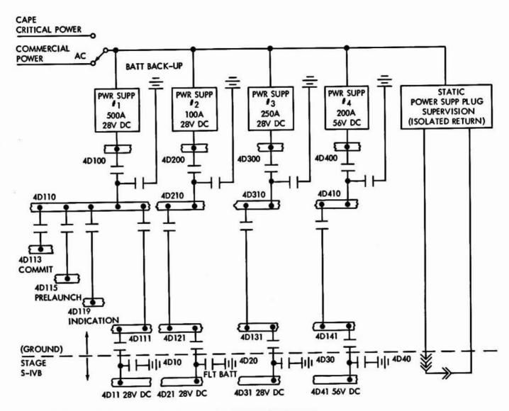
NOTE: POWER TRANSFER IS ACCOMPLISHED USING MOTORIZED SWITCHES
