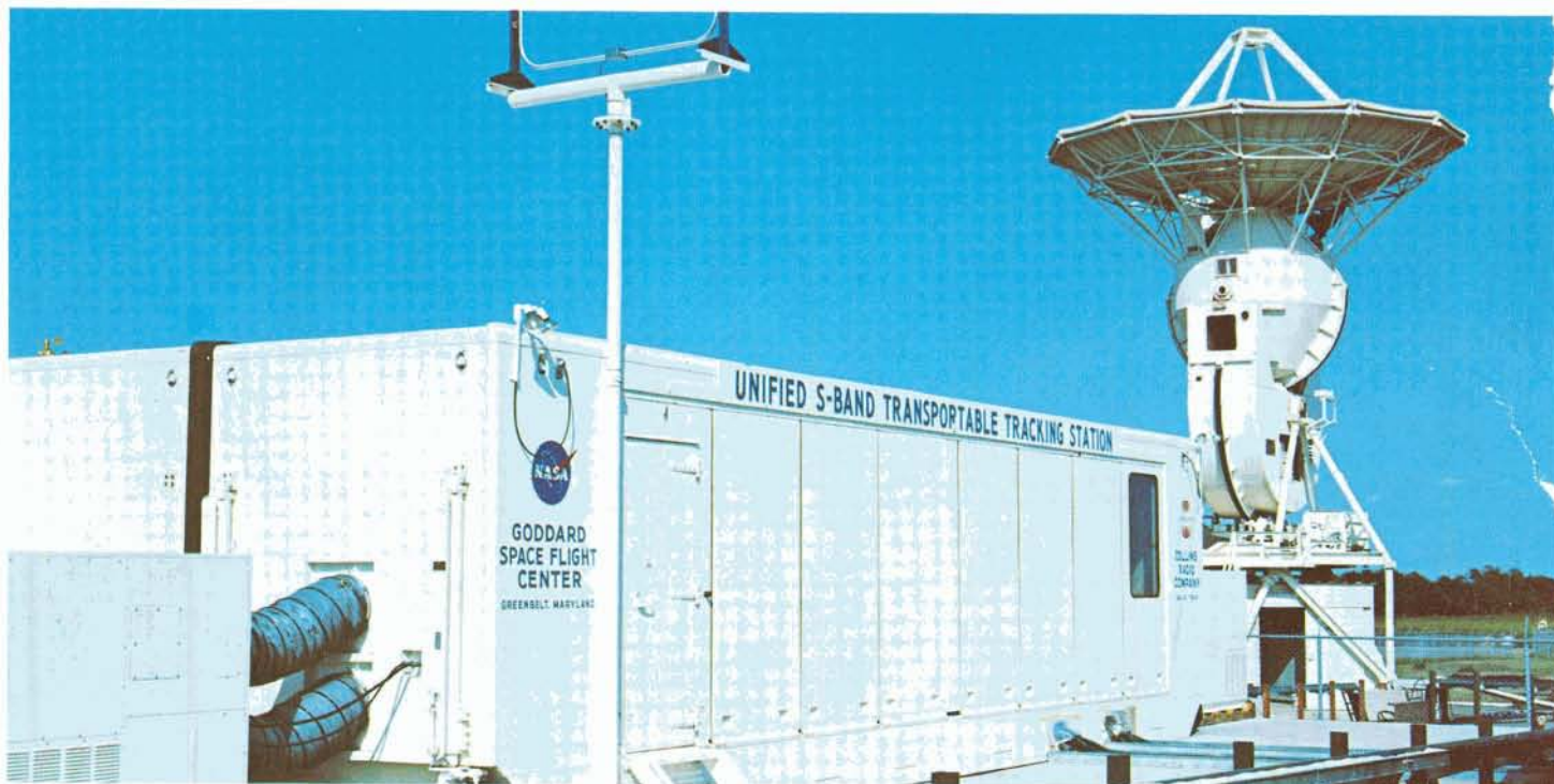
This transportable unified S-band tracking and communication station is being used in the lunar landing program. Station is one of 15 built by Collins for NASA's Goodard Space Flight Center, which is responsible for the worldwide Manned Space Flight Network.
