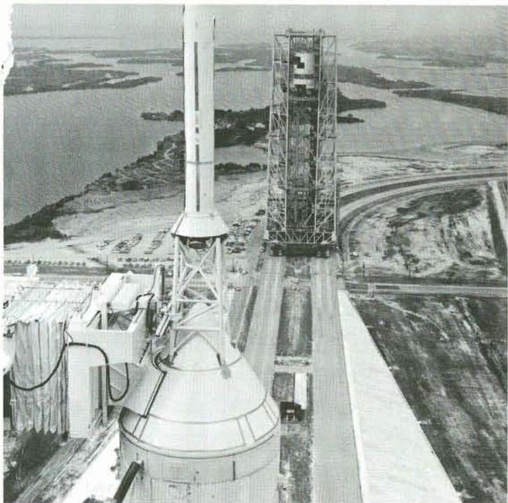
View from atop Apollo 4 before launch from Kennedy Space Center shows approaching mobile service structure, which is used to ready launch vehicle and spacecraft for flight.
