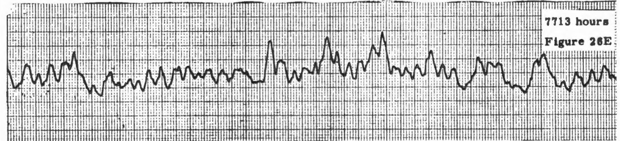
Figure 26. Ball Beat Frequency Traces for Wheel CR-113B
